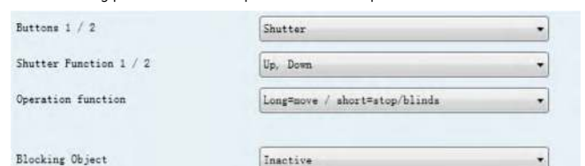
Figure 7: Double key curtain parameters
