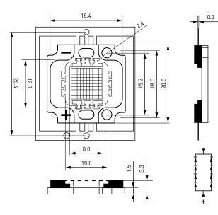
Note: all dimensions in mm tolerance is +0.1mm unless otherwise noted
