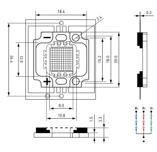
Note: all dimensions in mm tolerance is +0.1mm unless otherwise noted
