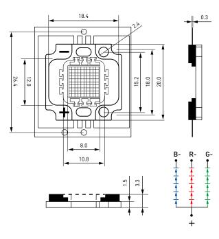
Note: all dimensions in mm tolerance is ±0.1mm unless otherwise noted.
