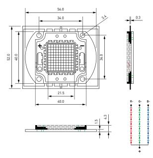
Note: all dimensions in mm tolerance is ±0.1mm unless otherwise noted.
