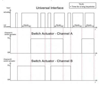
The following picture shows the long/short press used together, long press open, short press close:
