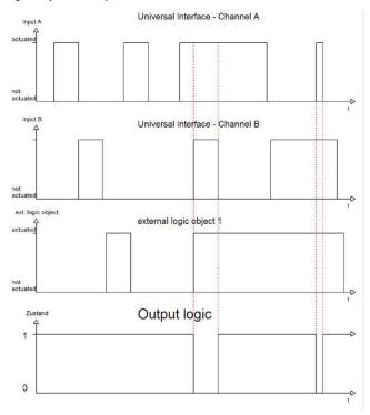
In the figure above, only when all three inputs are 1, the result of And operation is 1, the output after reverse is 0, And the output at other times is 1.
